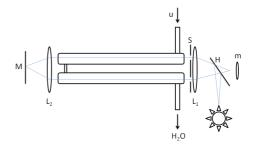
Fig.7. Fizeau's experiment on the propagation of light through moving water. m, microscope with micrometer; H, half-silvered mirror;  $L_1$ ,  $L_2$ , converging lens; S, slits; M, mirror.
